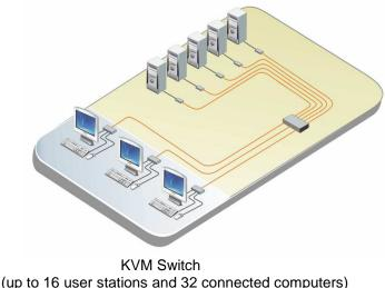
Cables... Cabling from the transmitters to Orion and from Orion to the receiver uses CATx solid wire (AWG24) cable or singlemode or multimode fiber cable. Cabling from the computers and the transmitter uses Rose Electronics DVI-CPU adapter cable. The KVM station's keyboard, DVI monitor, and mouse connect directly to the receiver.
